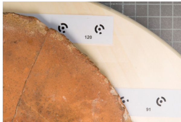
Figure 3. Image of the data collection where the plaque is located on the rotating platform (with coded targets) and this in turn on the reproduction table (grey grid) is observed.
