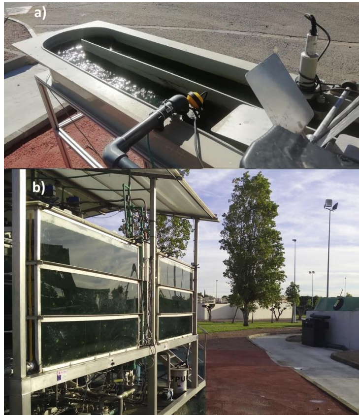
Figure 2. Intensive microalgae cultivation systems: a) Pilot-scale raceway pond; b) Pilot-scale closed photobioreactor.
