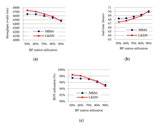
**Figure 9.** Performance of LKDN (Look-Downstream) and MBS6 (Minimum Batch Size 6) over different BP utilization levels in terms of (**a**) throughput, (**b**) production lead time, and (**c**) BOT (bottleneck) station utilization.
