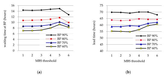
**Figure 8.** Performance of different MBS levels batch sizes in the MBS control in terms of (**a**) waiting time at BP station and (**b**) system lead time.
