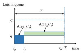
**Figure 2.** Changes in waiting time when the lots are loaded at time  $t_1$ . The saved wait time is  $\text{Area}_2(t_1) - \text{Area}_1(t_1)$ .
