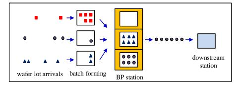
Figure 1. Schematic representation of a batch processor (BP) station with multiple batch processors.
