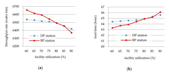
**Figure 7.** Performance compared over different BP and DP utilization levels in terms of (**a**) throughput rate per nine months and (**b**) system lead time.
