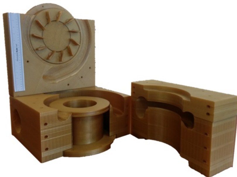
Figure 13. 3D printed scaled turbine.
