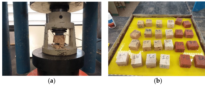
Figure 21. Analyses carried out in the laboratory of the Universitat Politècnica de València: (a) Determination of compressive strength; (b) determination of water absorption by capillarity.
