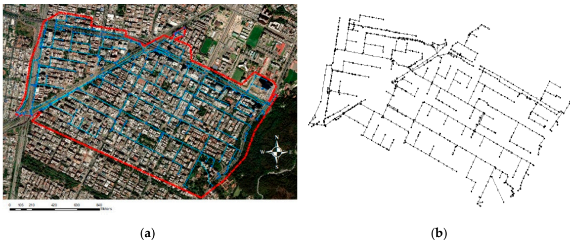
Figure 5. (a) Location of Southern Chicó Network. (b) Storm Water Management Model (SWMM) for Southern Chicó Network.
