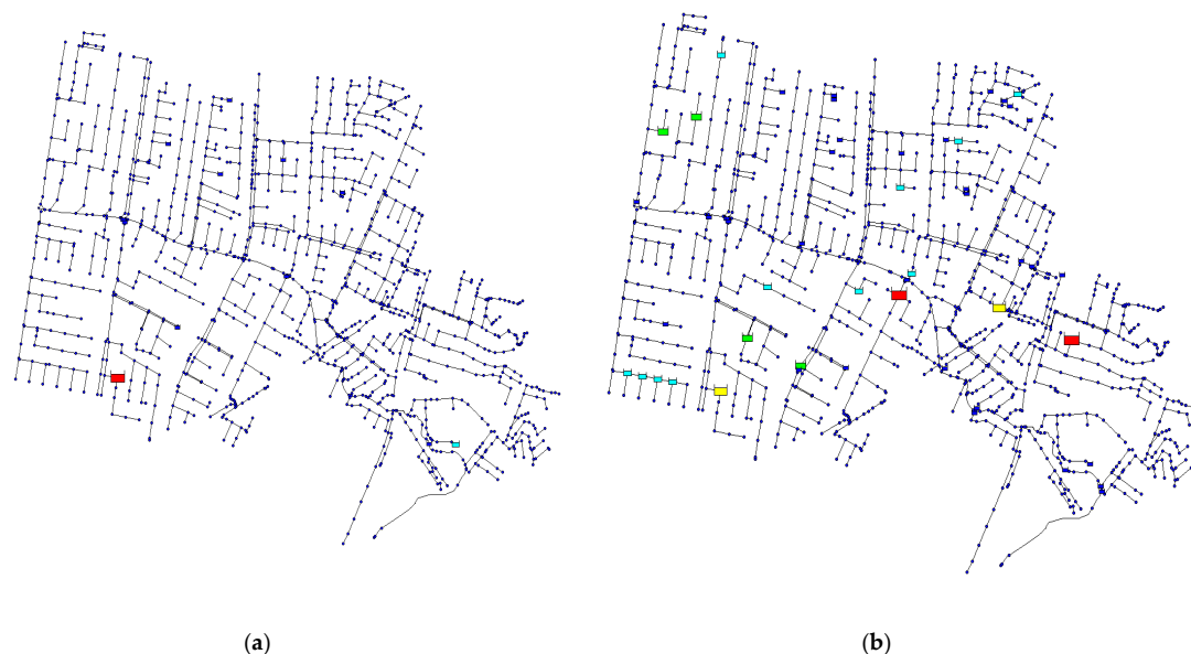
Figure 11. Results for the stormwater tank locations using OptiTank. The colors represent the size of the stormwater tank where red is the largest followed by yellow, green and cyan. (a) Results considering the current rainfall scenario. (b) Results considering the Climate Change effects on rainfall.
