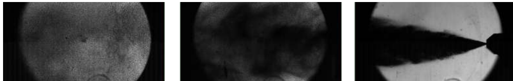
Figure 23: Example of the images acquired with the Schlieren technique for the NewNozzle with Novec1230 at 2.5 MPa and back pressure of 0.1 Mpa.
