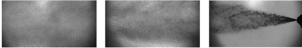
Figure 21: Example of the images acquired with the DBI technique for the NewNozzle with water at 2.5 MPa and back pressure of 0.1 Mpa.
