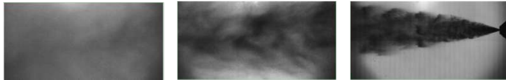
Figure 22: Example of the images acquired with the DBI technique for the NewNozzle with Novec1230 at 2.5 MPa and back pressure of 0.1 Mpa.
