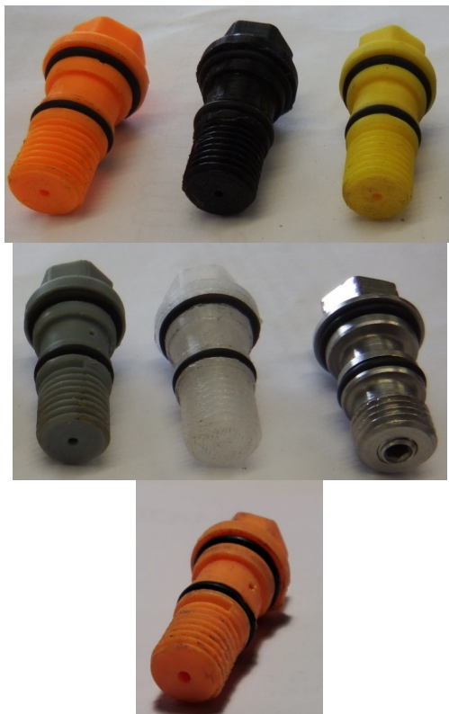
Fig. 3 STK-ZZ-2 nozzles: 1-5 printed vertically from Z-ULTRA, Z-HIPS, Z-ABS, Z-PETG, Z-TRANSPARENT, 6 - commercial, made of metal, 7 - printed horizontally from Z-ULTRA
