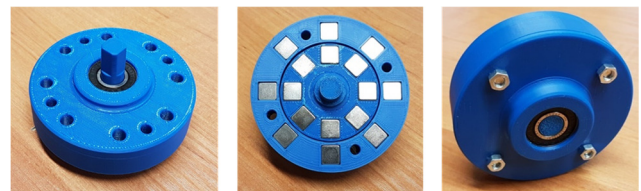
Fig. 14 Physical model of a single-row cylindrical clutch Source: [6].
