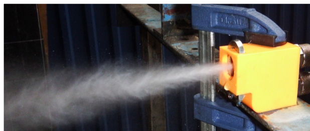
Fig. 9 Test of the spraying stream of the plug-in nozzle
