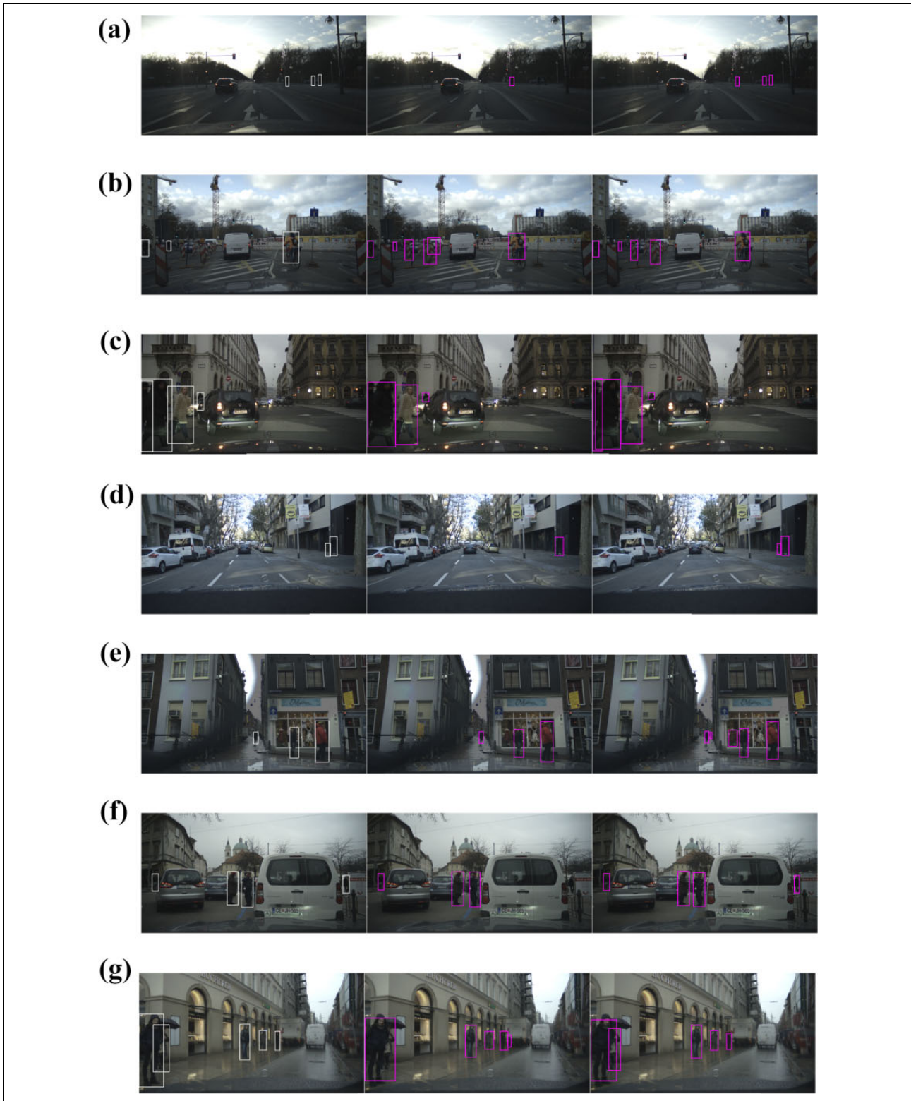
Figure 7. Pedestrian detection for the original YOLOv3 and the YOLOv3 for pedestrians on the ECP dataset: (a) berlin_00414, (b) berlin_00436, (c) budapest_00859, (d) barcelona_01293, (e) amsterdam_01078, (f) ljubljana_01051 and (g) hamburg_00681. From left to right: ground truth, original YOLOv3 and single class YOLOv3. YOLO: You Only Look Once; ECP: EuroCity Persons.
