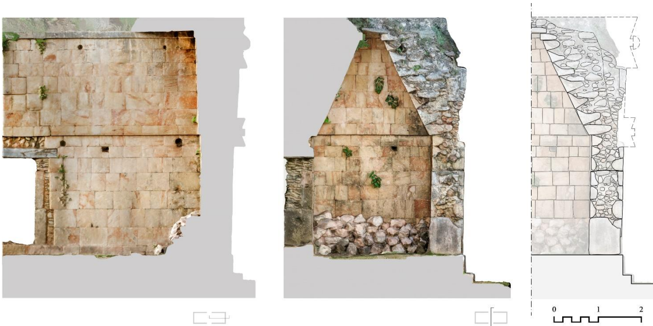
Figure 8. Scaled orthophotos and constructive section of room 1 of the House of the Turtles obtained from the photogrammetric model.
