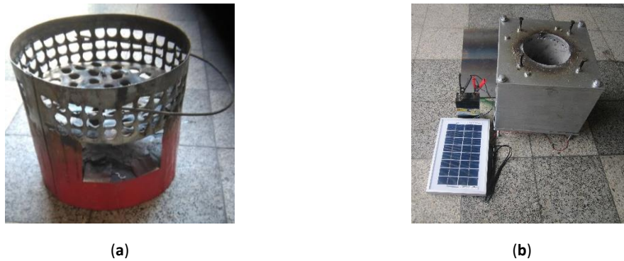
Figure 2. Cooking stoves. a) Traditional cookstove, TCS. b) Improved Cookstove Gasifier, ICS-G
