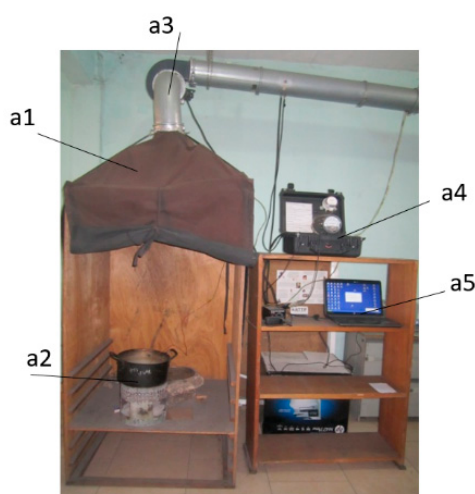
Figure 4. Portable Emission Monitoring System (PEMS).
