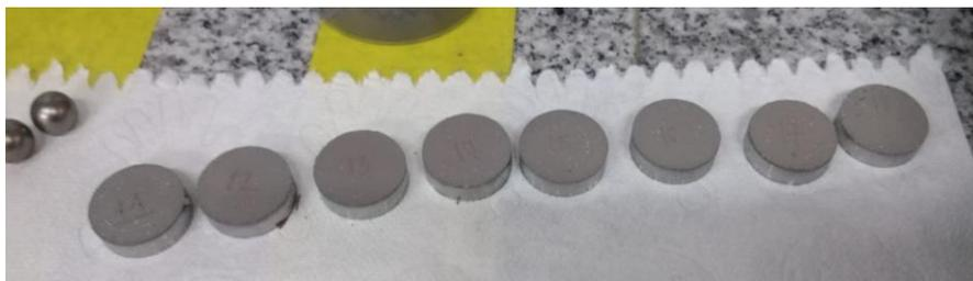
**FIGURA 23. PROBETAS DE BE COMPACTADAS A 600 MPA.**
