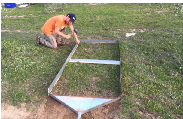
Figure 10: Soil erosion plot (2 m 2 ) at the Sierra de Enguera experimental station.
