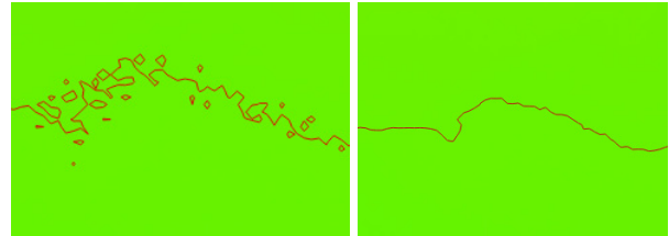
Figure 13: SAGA "simple filter" process on original DTM model in area with a lot of noise and generated smoothing.
