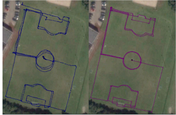
Figure 4: Dual-frequency test at the European Space Technology Centre (ESTEC). Samsung S8 (left), Xiaomi Mi-8 (right). Source ESA.
