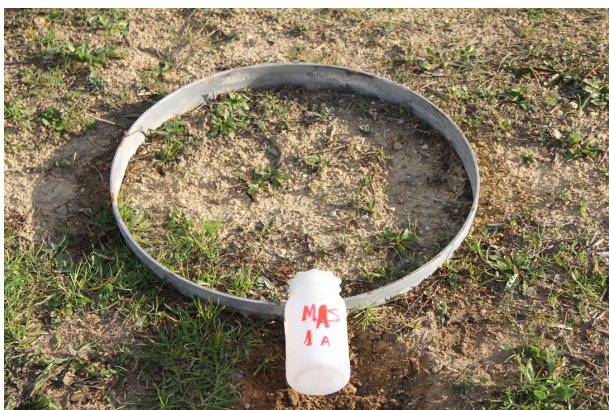
Figure 9: Example of rainfall simulation plot (0.25 m 2 ).
