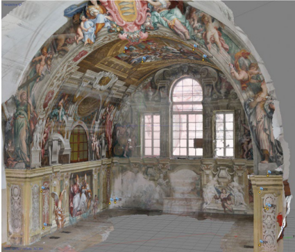
Figure 2. Frescoed apse in the former church of Saints Gerolamo and Francesco Saverio. Elaboration of the photoscan survey. Source: (MARS C 2019)
