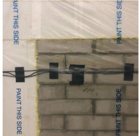
Figure 3a. DWB specimen wall prior to testing. Figure 3b: Wall detail. Wall has been instrumented, mounted in frame, and frame is clamped to climatic chamber.
