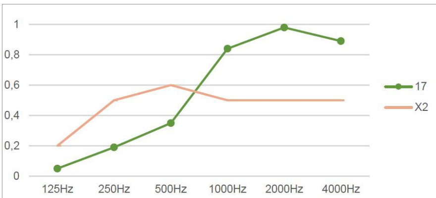
Figure 6. Absorption coefficient spectrum of the upholstered wall frames (before -green- and after -pink- RSM application).
