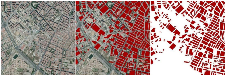
Figure 1. Aerial photography as a reference, vector dataset 1: 50,000 cartography superposition. Source: the authors
