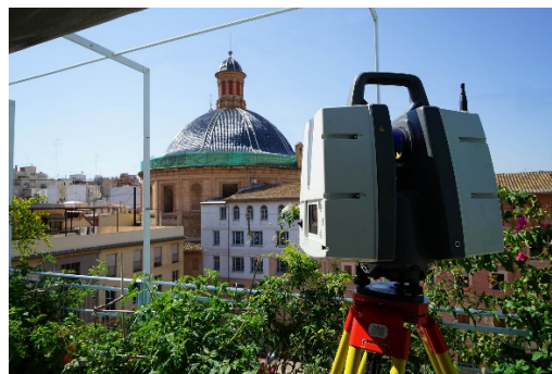
Fig. 9 Data collection from nearby buildings by means of a 3D laser scanner. Source: Rodríguez-Navarro & Gil-Piqueras
