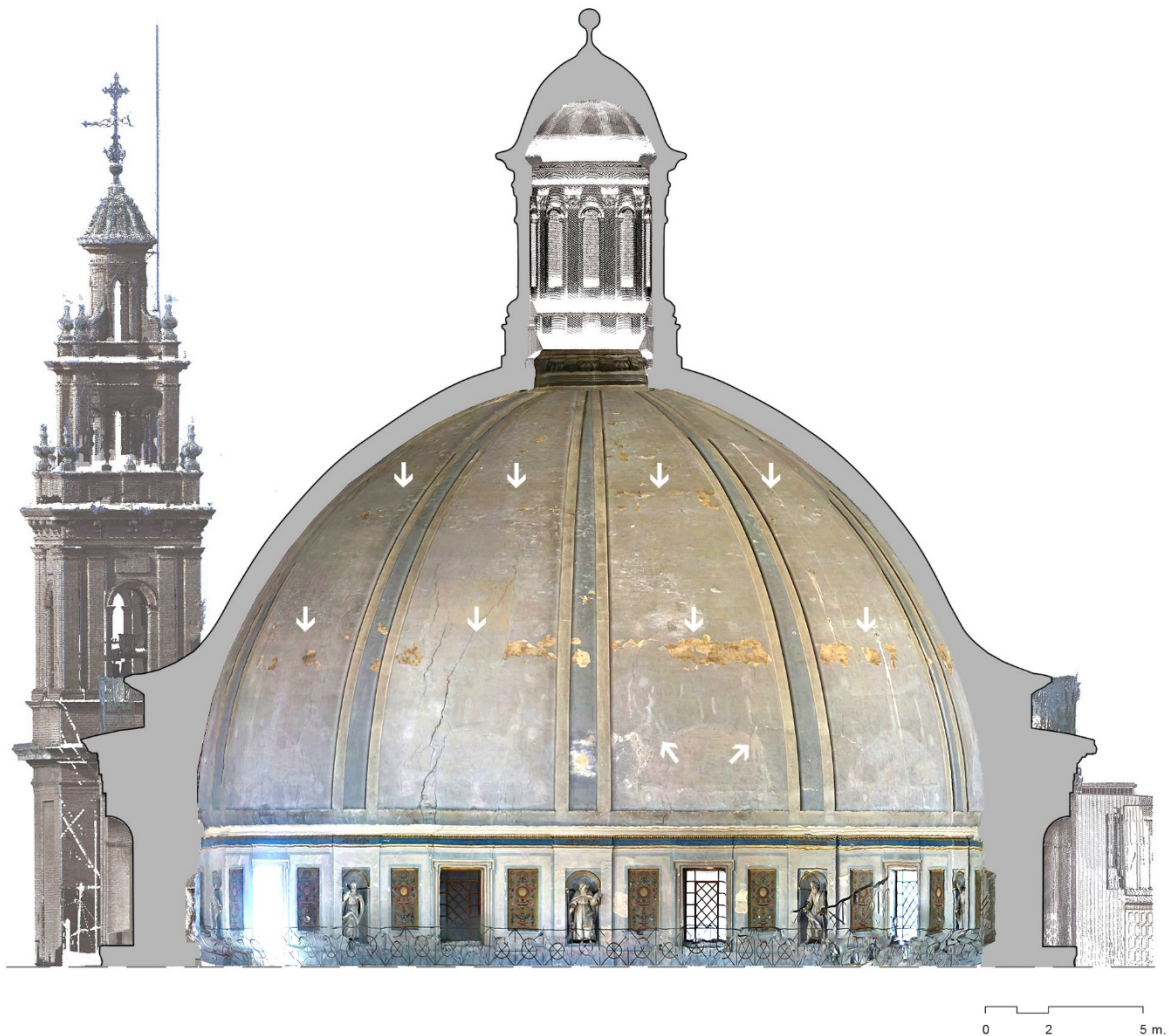
Fig. 11 Photogrammetry of the dome over the 3D laser scanning point cloud. Visualization of damage due to metal rings and presence of relieving arches. Source: Rodríguez-Navarro & Gil-Piqueras
