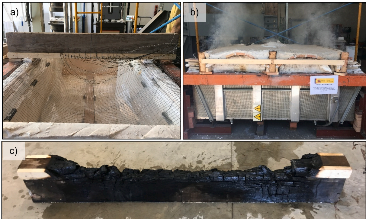
Fig. 7. Experimental test: (a) furnace and timber elements instrumentation; (b) fire test; and (c) charring state of the timber joist after the test.
