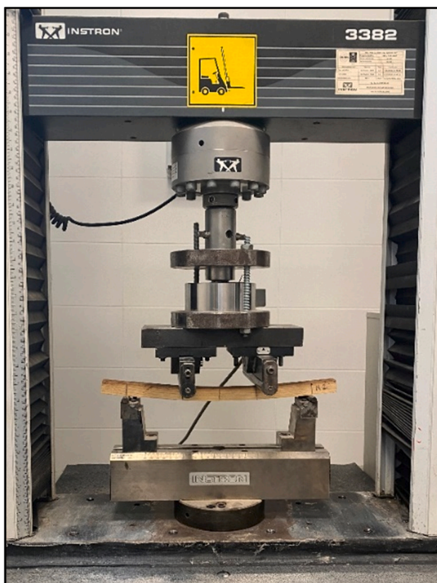
Fig. 14. Four-point bending test carried out.
