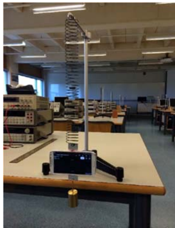
Figure 2. “Spring+mass+smartphone” oscillating system.
