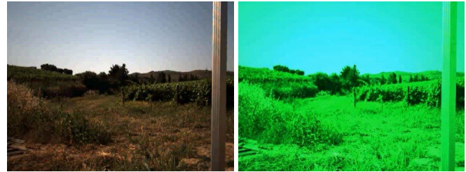
Fig. 2. Effects of ambient temperature on a stereo camera: (a) Temperature below 30^{\circ} ; (b) Temperature above 40^{\circ} C causing the loss of the red color component in the RGB CMOS sensor.
