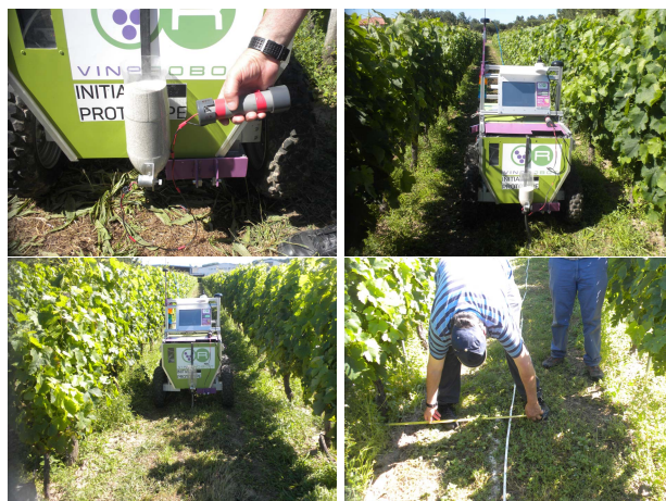
Fig. 6. Evaluation of guidance performance with lime-marked trajectories.
