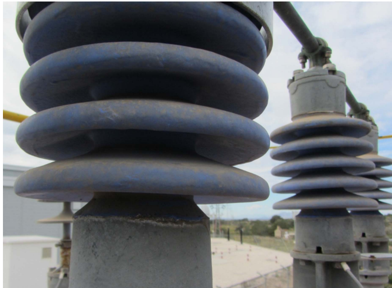
Figure 1. Coated insulators in the test panel.
