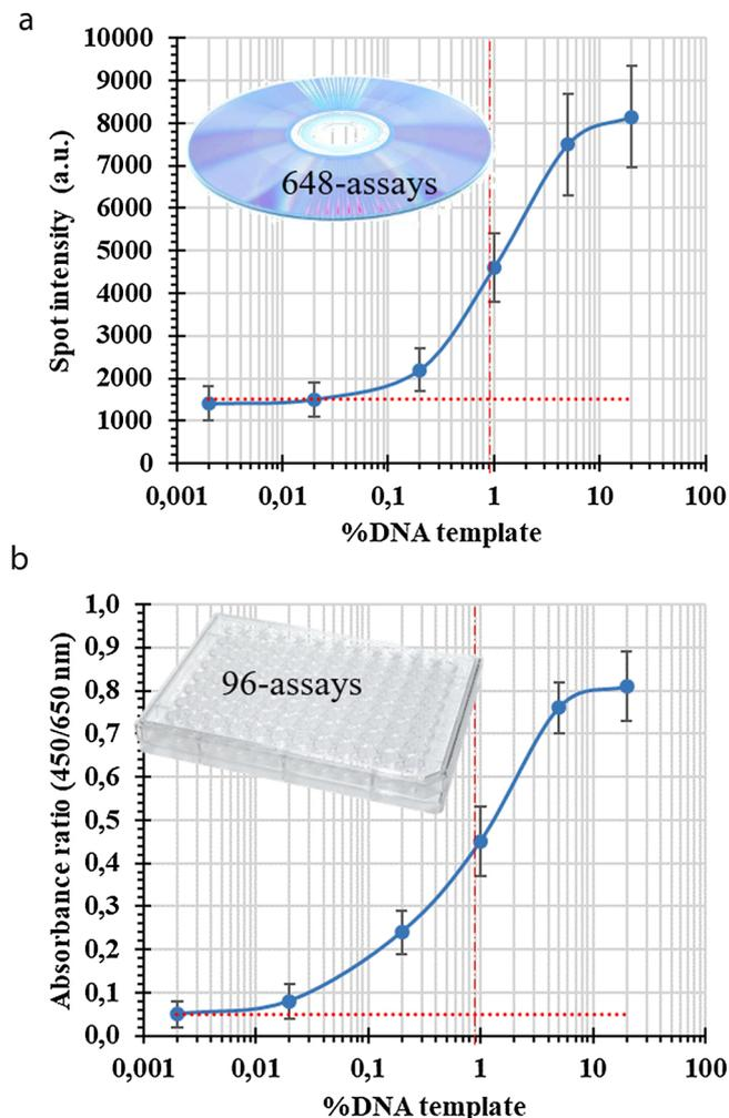
**Fig. 4.** Comparison of GMO detection capability based on multiplex-RPA/DVD biosensing (a) and the single PCR-ELISA method (b). Dotted lines indicate the corresponding detection limit and the labelling limit as regulated in the EU (0.9 % of GMO).
