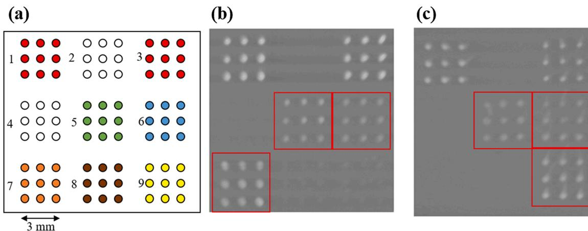
**Fig. 5.** Application to the analysis of certified reference materials. (a) Array layout. 1: positive control (hybridisation), 2: negative control (hybridisation), 3: positive control (staining), 4: negative control (staining), 5: terminator T-nos, 6: promoter P-35S, 7: soya bean, 8: potato, 9: corn. (b) DVD image for soya bean RRS 5%. (c) DVD image for corn Bt-11 5%.
