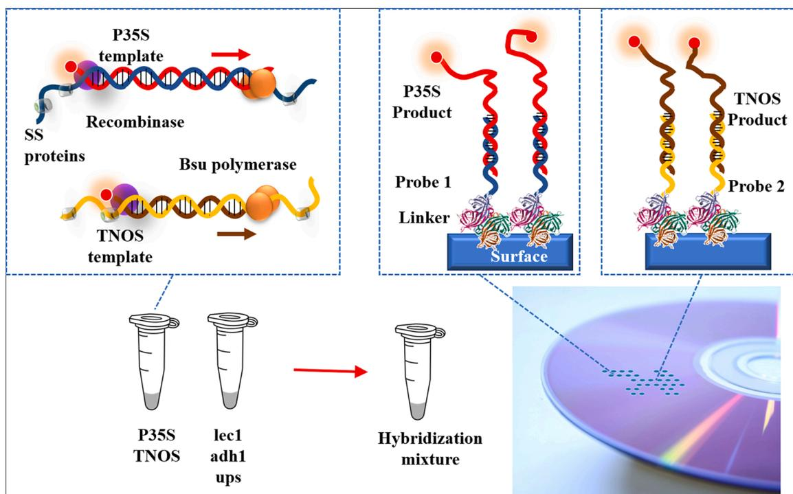
Fig. 1. Scheme of the assay for GMOs detection based on multiplex RPA amplification (left) and hybridisation assay in the array format (right).
