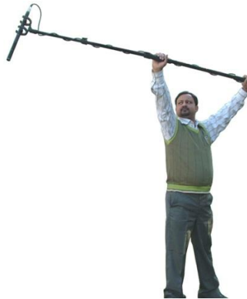
51. Shotgun microphone installed on a boom.
