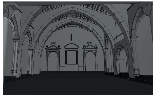
Fig. 9. HBIM modeling of the current phase of La Sang. Picture, point cloud and BIM model (Source: Moral, Sergio).
