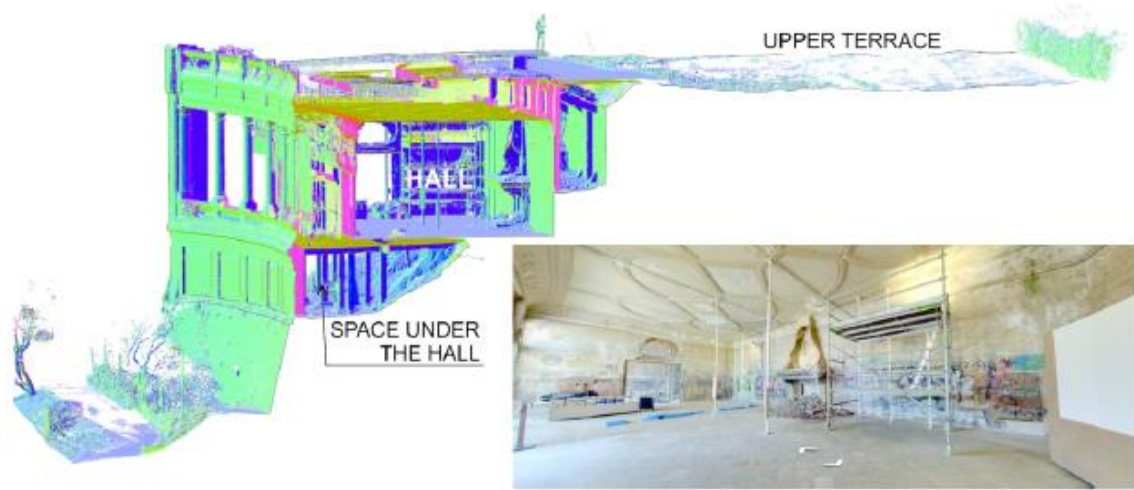
Fig. 2. Three-dimensional image of the investigated area. Photograph of the building hall, main built body, damaged not only by water inflows from the roof but also by underground flows coming from the upper terrace.
