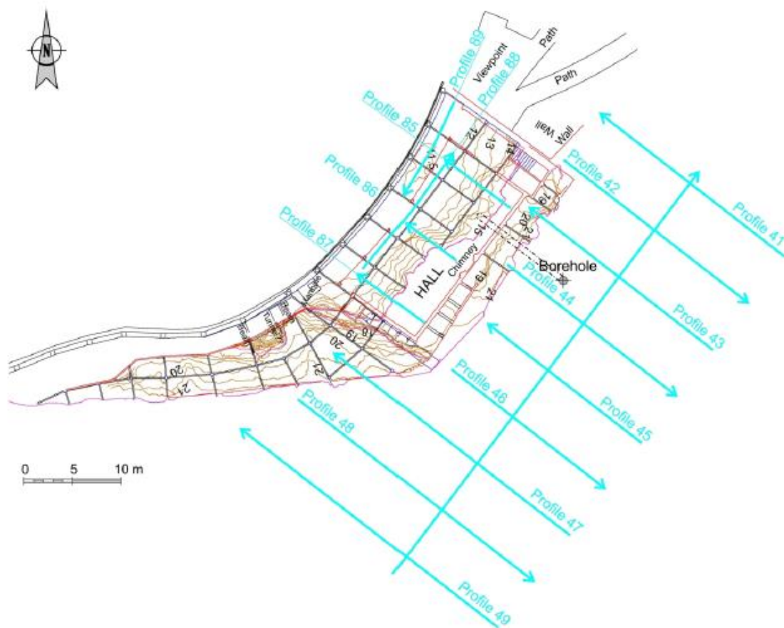
Fig. 3. Plan of the galleries. Location of the GPR profiles (blue lines).
