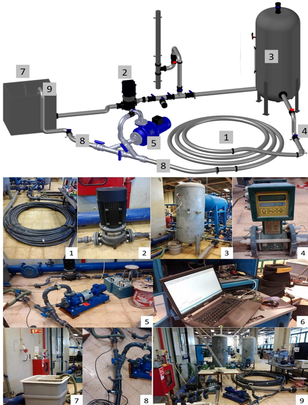
Figure 3. Experimental set-up of the PAT pilot station: (1) HDPE conduction; (2) recirculation pump; (3) air vessel; (4) flowmeter; (5) PAT; (6) picoscope and acquisition system; (7) regulation; (8) pressure transducers; and (9) hydrant.
