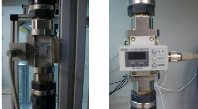
Figure (8.10): Two different flow meters are used to measure the jet flow rate
