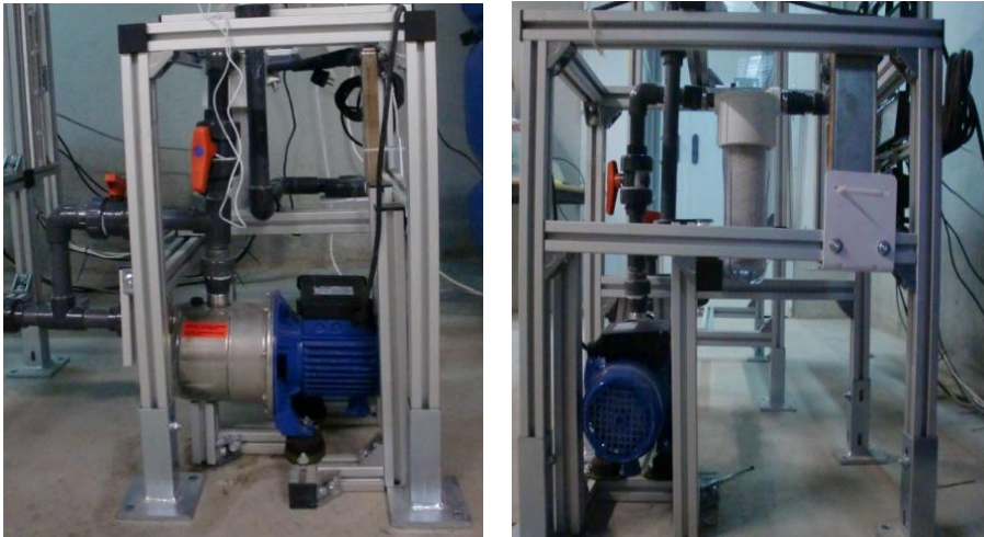
Figure (8.4): Water re-circulation and skimming system
