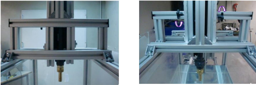
Figure (8.6): Mechanism to support the nozzle vertically
