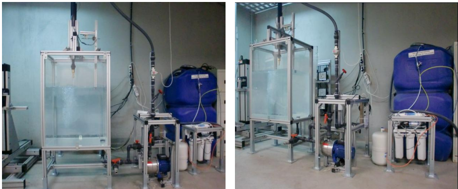
Figure (8.2): Pictures showing the experimental set-up of the plunging jet system
