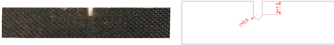
738 Figure 1. Detail of “U” type notched samples for Charpy test to evaluate the impact 739 strength of hybrid composite laminates with different basalt/flax plies with a partially 740 bio-based epoxy resin.
