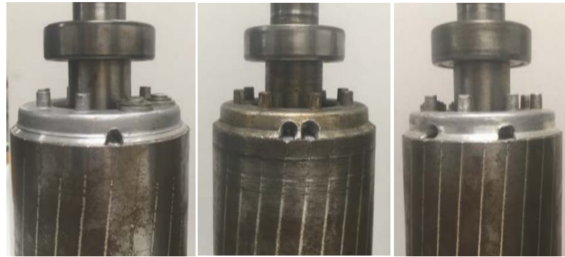
Figure 11. Tested rotors with faulty cages: one broken bar ( left ), two consecutive broken bars ( centre ) and two non-consecutive broken bars ( right ).
