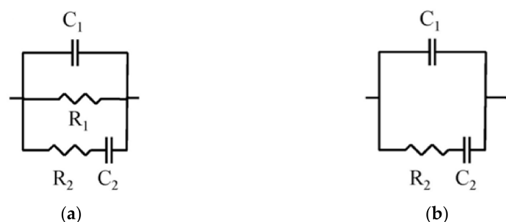
Figure 2. (a) Equivalent circuit used for fitting the impedance spectra obtained using the contacting method. (b) Equivalent circuit used for fitting the impedance spectra obtained using the non-contacting method.
