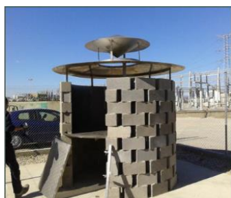
Figure 2. Self-made burner to obtain rice straw ash (RSA).
