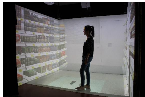
Fig. 3. Low-cost CAVE powered by the KAVE software.
