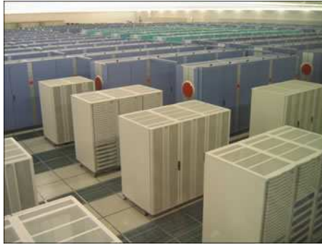
Figure 2.2: The Earth Simulator massive parallel processors. 640 vector processors (8 pipelines each one). 640x640 switch crossbar. 16 GB/s of Bandwidth.
