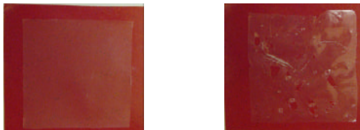
Photo 3. EVOH32/ionomer blend before (left) and after (right) retorting in autoclave
