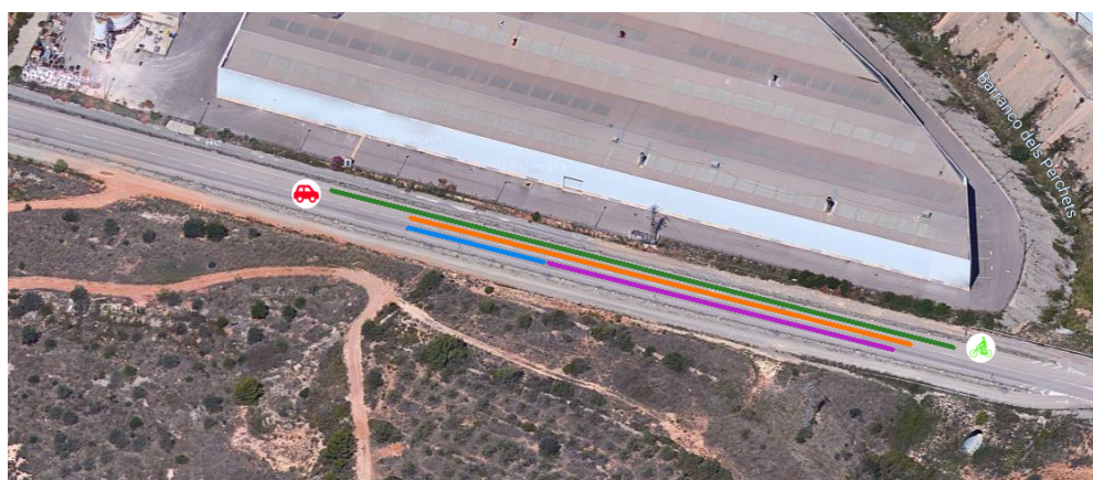
Figure 18. Image with distances for the worst case (car and bicycle in opposite directions with a relative speed of 90 km/h). The green line is the alarm threshold (150 m) the orange line shows the distance when the alarm pops up (121 m); the blue line is the car breaking distance (31 m); and finally, the purple line is the remaining distance when the two vehicles are stopped (88 m). Note that the reaction time in the experiment is quite reduced because the driver is waiting for the alarm.
