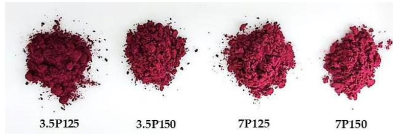
Figure 2. Appearance of studied beetroot powder samples: 3.5P125 or 3.5P150, powder with 3.5% of pea protein concentration spray dried at 125 or 150 °C, respectively; 7P125 or 7P150 powder with 7% of pea protein concentration spray dried at 125 or 150 °C, respectively.
