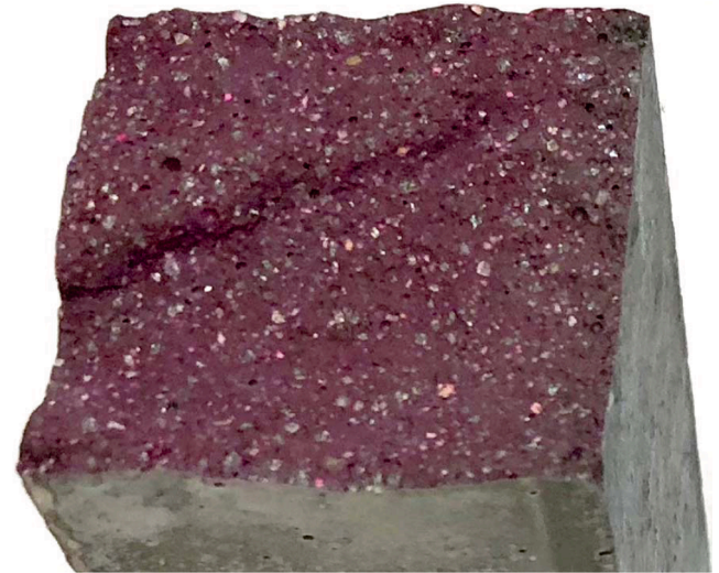
Fig. 7. Phenolphthalein method in concrete UH-0F-20 at the age of 1 year.
