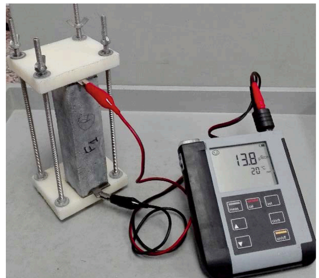
Fig. 2. Measuring conductance in prismatic specimens.
