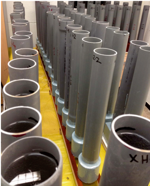
Fig. 1. Water tank with chlorides placed on the specimens.
