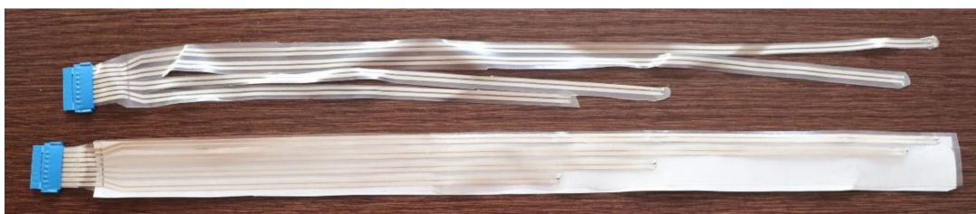
Figure A6. Final prototype. On the bottom, a complete multisensor; and on the top, a multisensor divided by sensors to facilitate its placement.
