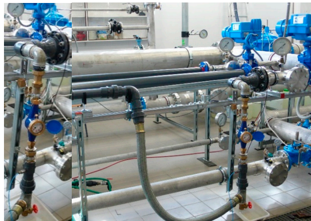
Figure 9. Water meter blocking laboratory test and detailed image of water meter test bench.
