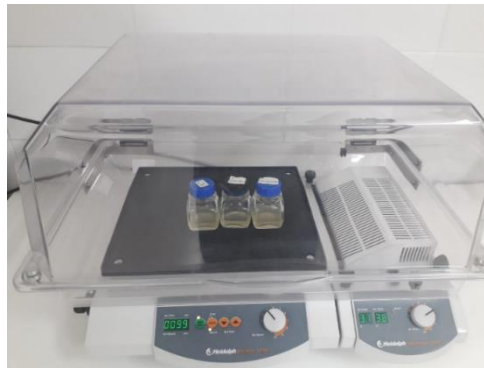
Figure 3.2. Rotary shaking incubator used in this work for growing of bacteria in liquid culture media.
