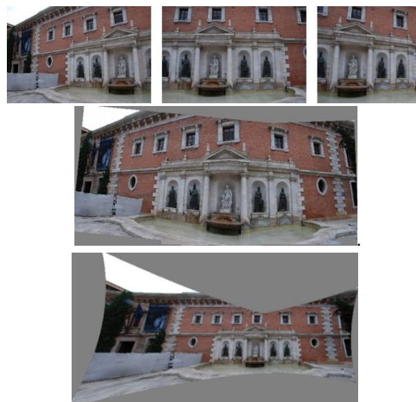
Fig.5: Facade of the Old University of Valencia in the Patriarch Square. Up: initial images with divergent directions. Middle: rigid-solid transformation over planar mapping. The photos result aligned to ensure that the overlapped content coincides with no deformation (no stretching or distortion). Below: general homography transformation over planar mapping. The images are linearly deformed so that the two laterals result aligned with the central, to recover the base-plane in the model
