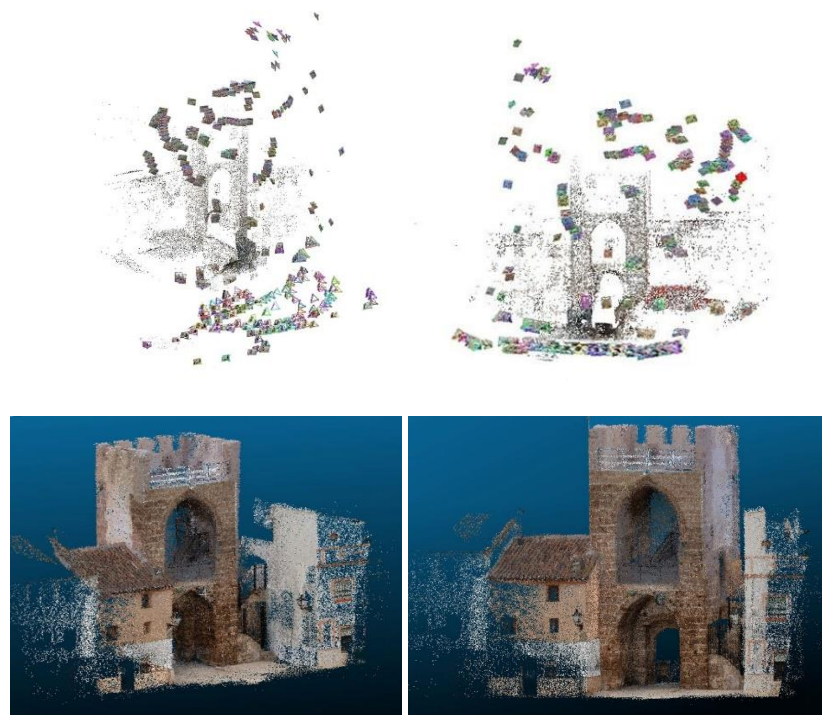
Fig.7: North Tower of Buñol’s Castle. Top: sequence of terrestrial and aerial shots describing respectively arcs and spirals. We have checked the effectiveness of these sequences, with nadiral and azimuthal angles of different signs, so that the orientations of the model are registered from all possible positions with enough redundancy, in order to optimize the SFD and Matching algorithms. (Cabanes & Bonafé, 2019). Bottom: interior views of the filtered 3D point cloud of the full model
