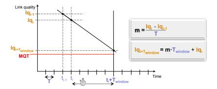
Figure 5.1: Link-quality-based adaptive packet replication technique
