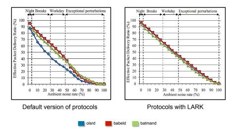
Figure 5.6: Effective Packet Delivery Ratio in proactive routing protocols
