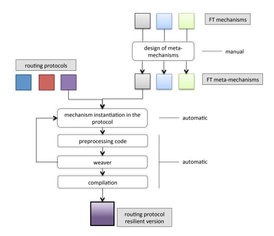
Figure 5.7: Transformation phases of the *fault tolerance meta-mechanisms* and routing protocols
