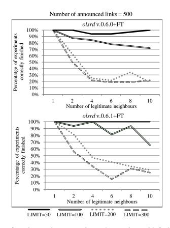
Figure 4.4: Percentage of survivor nodes to experimental campaigns with fault tolerance mechanism enabled
