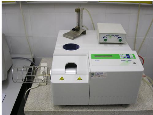
**Figura 42 Termobalanza Mettler Toledo TGA850.**
