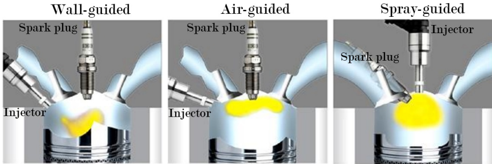
Figure 2.7: Different combustion systems in a GDI Engine. Adapted from [21].
