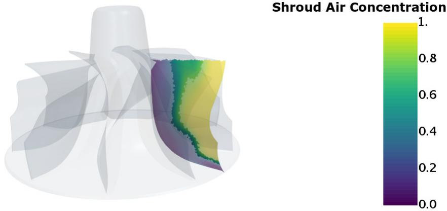
Figure 5.24: Shroud air concentration in a section at the middle of a rotor channel.
