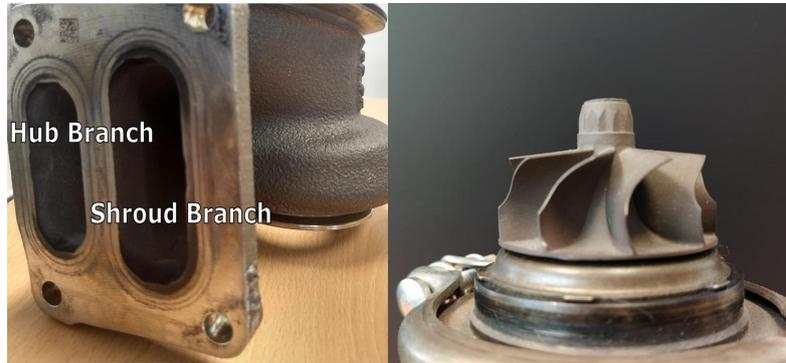
Figure 3.1: Twin-entry turbine entries and rotor
