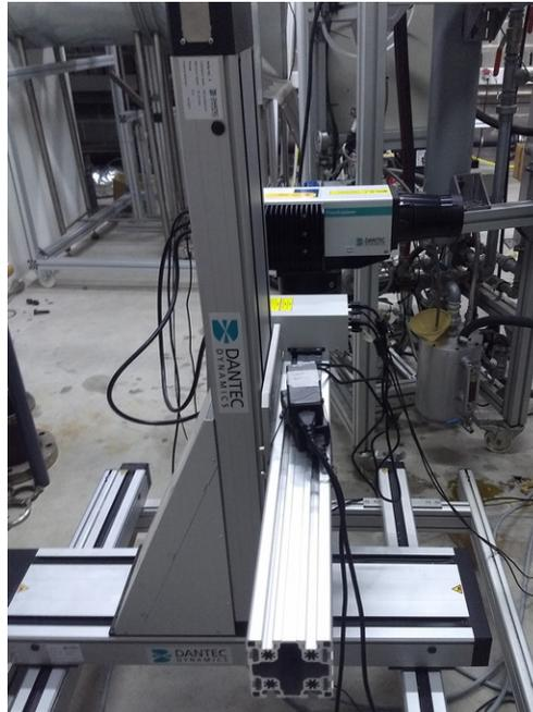
Figure 3.7: LDA system and traverse system.
