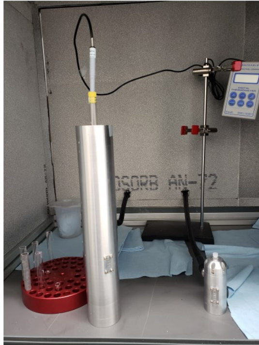
Fig. 1: Multipoint reentrant cavities employed to determine the permittivity spectrum of low-loss liquid and powder geomaterials.
