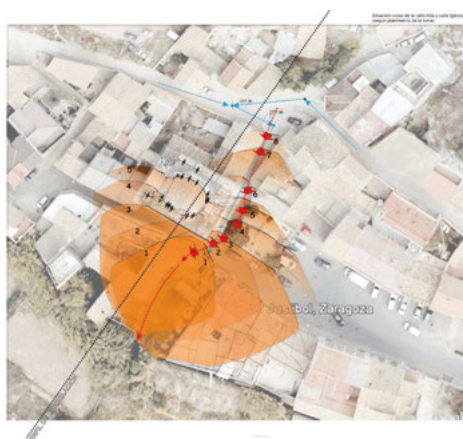
Fig. 2. Location plan. Situation and morphological analysis of the cracks on aerial photography (Source: Investigation report for the assessment of problems in the subsoil of the justibol church (Zaragoza) , 2014).
