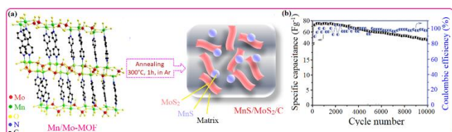
Figure 14. (a) Synthesis of MnS/MoS 2 /C electrode, (b) cyclic stability and Coulombic efficiency of MnS/MoS 2 /C electrode. Reproduced with permission from Ref. [57] Copyright 2018, The Royal Society of Chemistry.
