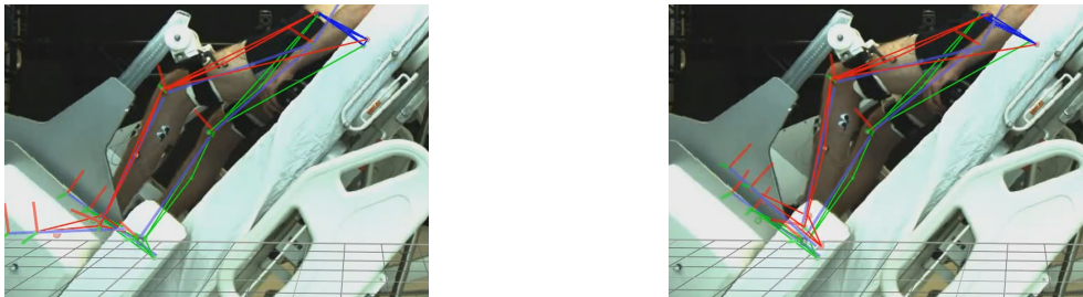
Figure 3.1: Overlay picture of Vicon Nexus and Video during maximum hip angle and two different options of moving the ankle joint: (a) only rotation and (b) actively lifting the sliding rail
