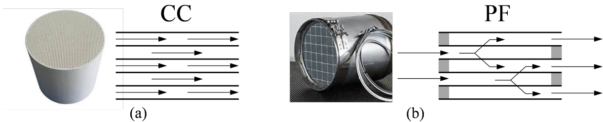
Figure 2: Monolith and flow pattern: (a) Catalytic converter (CC); (b) Particulate filter (PF).
