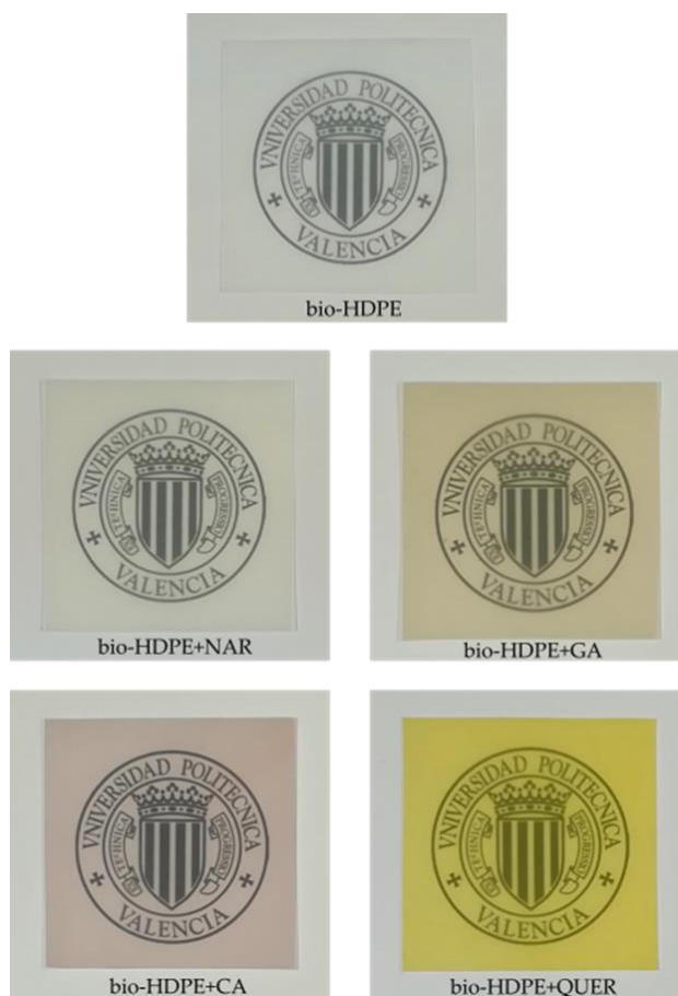
Figure IV.1.1.2. Visual appearance of the thermo-compressed bio-based high-density polyethylene (bio-HDPE) films containing naringin (NAR), gallic acid (GA), caffeic acid (CA), and quercetin (QUER).
