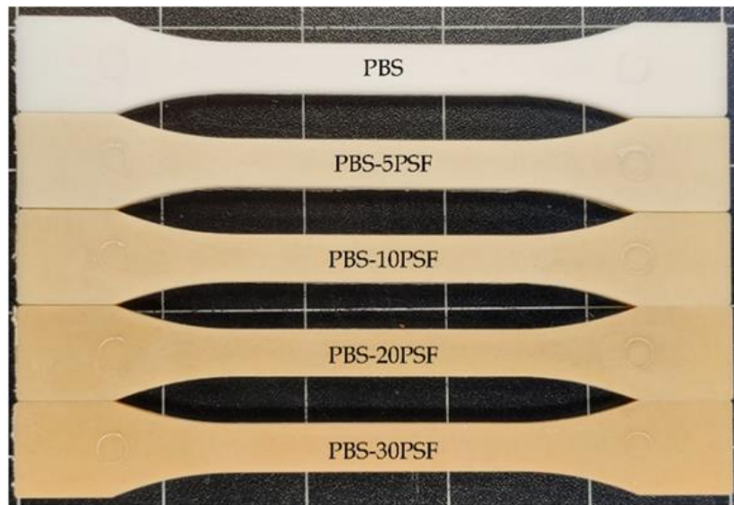
Figure IV.2.2.2. Visual appearance of the injection-molded pieces of poly(butylene succinate) (PBS)/pistachio shell flour (PSF) compatibilized with poly(butylene succinate) grafted with maleic anhydride (PBS-g-MAH).
