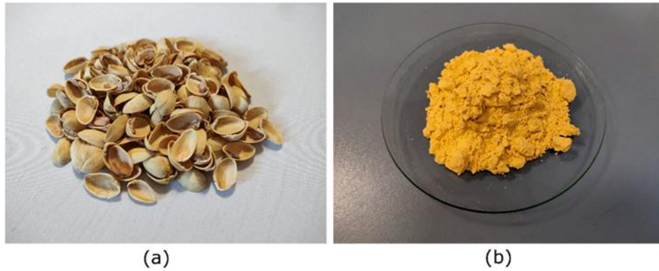
Figure IV.2.2.11. (a) Pistachio shells; (b) Resultant pistachio shell flour (PSF) after milling and sieving.
