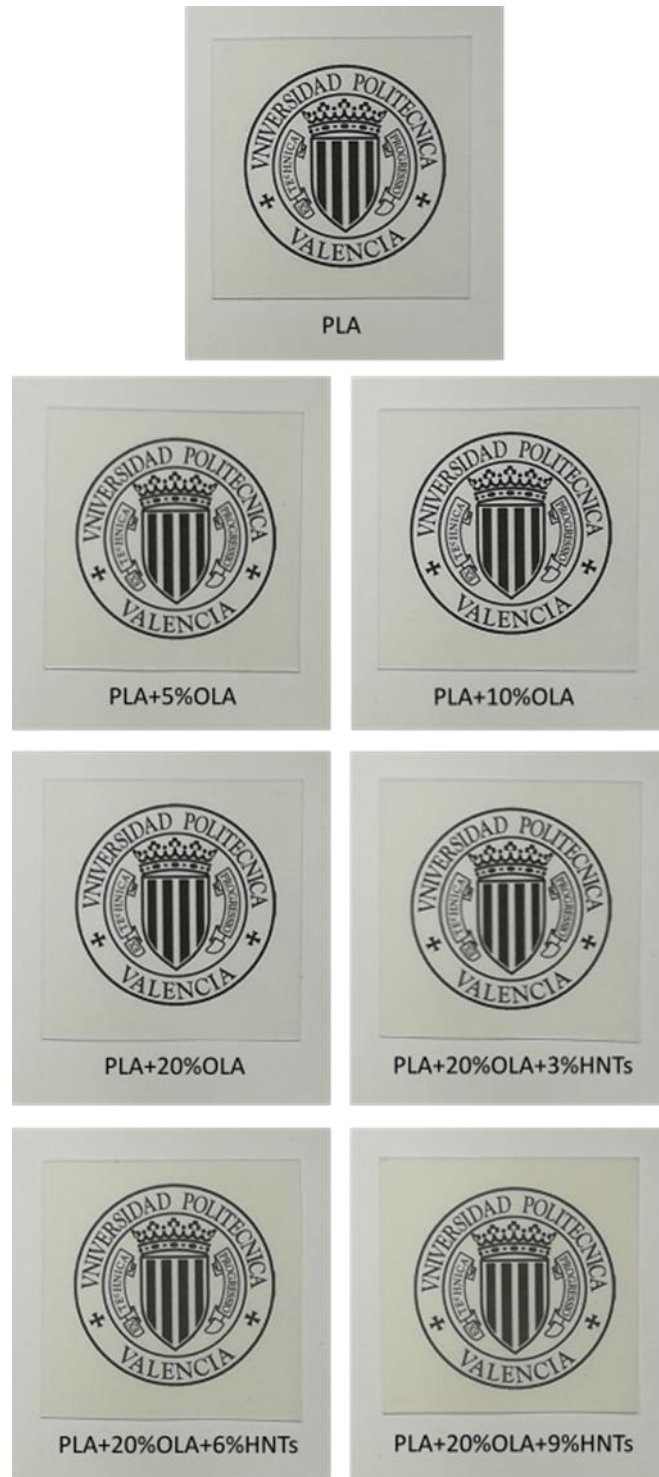
Figure IV.2.1.1. Visual aspect of the polylactide (PLA)/oligomer of lactic acid (OLA)/halloysite nanotubes (HNTs) films.
